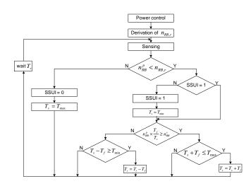
Figure 5. Flow chart of proposed sensing algorithm.
