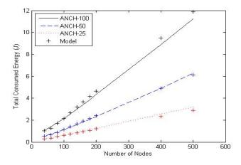
Fig. 7: Accuracy of the model comparing against simulation results for three values of MNumber, MNumber = 25, 50, and 100 messages per round.
