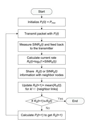
Figure 2. Flow chart of proposed BiTPC algorithm.
