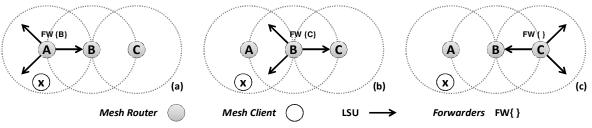
Figure 2. Implicit, positive acknowledgement mechanism.
