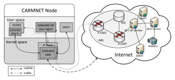
Figure 1: Interactions between CARMNET components.
