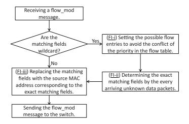
Figure 6. Summarized process of flow entry installation.
