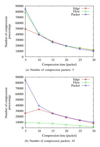
Figure 7. Effect of compression time: Number of compression processings
