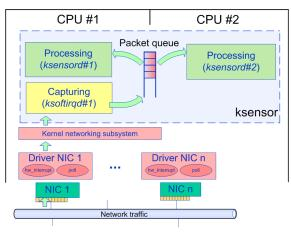
Figure 4. Execution instances in Ksensor with two processors and one NIC.
