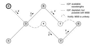
Figure 5. Recovery options for lightpath C perceived by the node 2.
