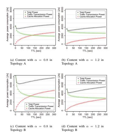
Figure 9: Power consumption of the network when the TTL value is changed
