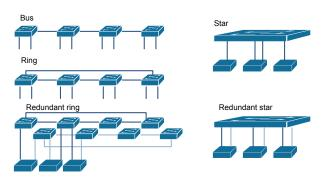
Fig. 2. Industrial Ethernet topologies
