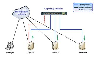
Figure 5. Network infrastructure to test the probes.
