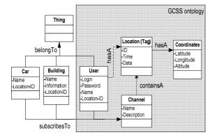
Figure 4. Overlay ontology used by GCSS
