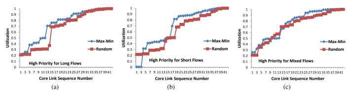
Figure 5: Core link utilization with high priority for (a) long flows (b)short flows (c)mixed flows
