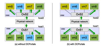
Fig. 3. Difference of treatment of a broadcast
