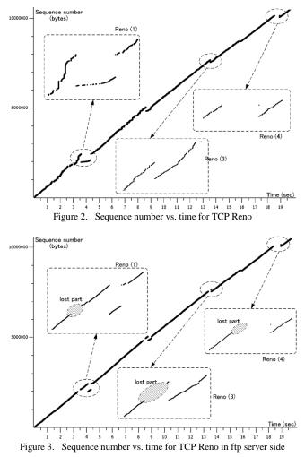
The other type is that for the fourth discontinuous section (Reno (4)) in the figure. Packets are lost in the end of continuous data sending and there is a time lag before the retransmission starts. We will examine the packet level behaviors of these two types in the next section.
