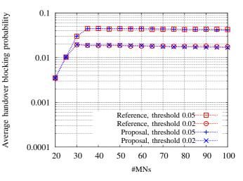
Figure 3. Handover blocking probability *versus* the number of MNs in Scenario 2.
