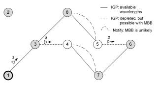
Figure 4. A Notify message is used to report the ingress node of each interrupted lightpath.
