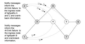
Figure 2. A Notify message is used to report the ingress node of each interrupted lightpath.
