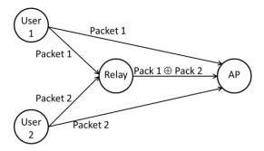
Figure 1. Wireless cooperative relay network with network coding.
