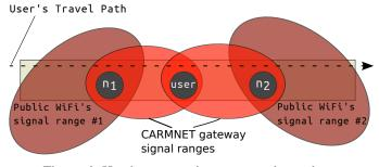
Figure 6: Handover experiment network topology.
