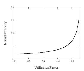
Figure 5. Normalized delay as a function of utilization factor,  $\rho$ , considering  $PER_{uap} = 0.3$  and  $PER_{ur} = PER_{rap} = 0.1$ .
