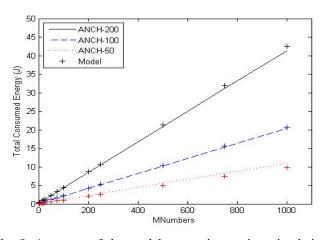
Fig. 8: Accuracy of the model comparing against simulation results for three networks with different number of nodes, N=50, 100, and 200.
