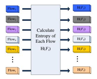
Figure 6. Measure entropy of each flow
