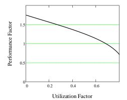
Figure 8. Performance Factor as a function of Utilization Factor, considering  $PER_{uap} = 0.4$  and  $PER_{ur} = PER_{rap} = 0.1$ .
