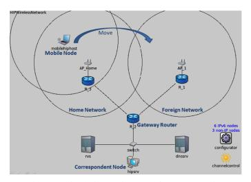
Figure 2: Simulation environment for HIP scenarios
