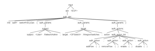
Figure 4. The AST tree for Listing 2 example
