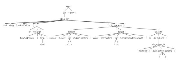
Figure 5. The AST tree for Listing 9 example
