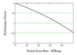
Figure 9. Performance Factor as a function of the Packet Error Rate in the link between the wireless user and AP,  $PER_{uap}$ , considering  $\rho = 0.8$  and  $PER_{ur} = PER_{rap} = 0.1$ .
