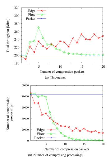
Figure 5. Effect of the number of compression packets
