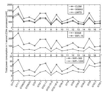
Figure 10: Total power consumption for C54x.
