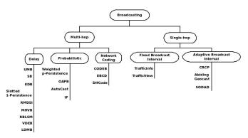
Figure. 1. Classification of broadcasts protocols in VANETs. Adapted from [6].
