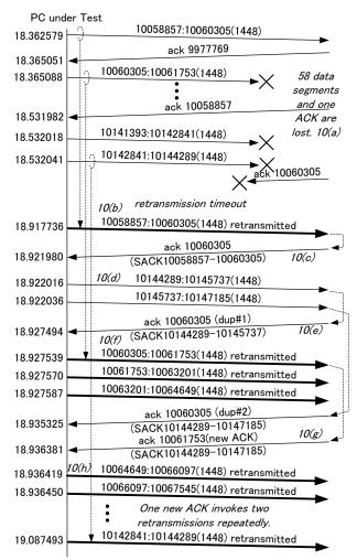
Figure 10. Timeline of segment exchanges at Reno (4)
