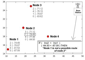
Figure. 4. Checking if node 1 can be a route to node 2.
