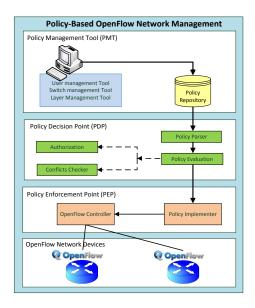
Figure 3. The Policy-Based OpenFlow Network Manager architecture
