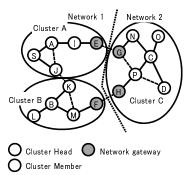
Figure 4: Network topology in heterogeneous MANETs.
