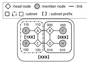
Figure 4: Result of group ID assignment procedure.
