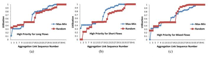
Figure 4: Aggregation link utilization with high priority for (a) long flows (b)short flows (c)mixed flows
