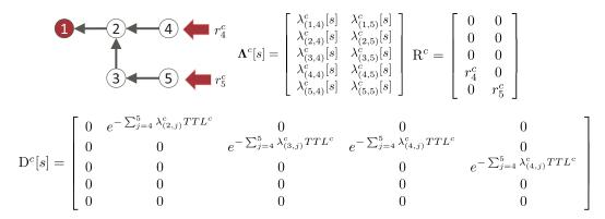
Figure 4: An example of matrices  $\Lambda^c$ ,  $\mathbf{R}^c$ , and  $\mathbf{D}^c$  for the request propagation on the delivery tree having origin 1
