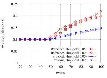
Figure 4. Latency versus the number of MNs in Scenario 1.
