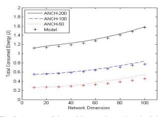
Fig. 5: Accuracy of the model comparing against simulation results varying network dimension for three networks with different number of nodes, N=50, 100, and 200.
