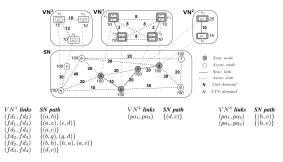
Fig. 5: Virtual networks mapping
