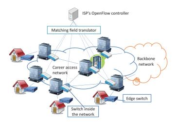
Figure 5. Deployment in a carrier access network.
