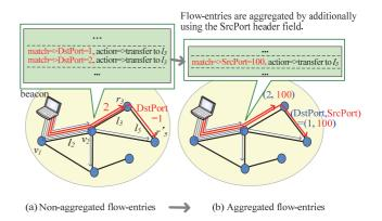
Figure 2. Flow aggregation of the flow-entries.
