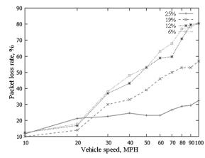
Figure 6. Packet loss rate while transmitting emergency message.
