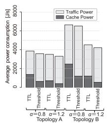
Figure 13: Power consumption for energy efficient TTL-based caching and threshold-based caching
