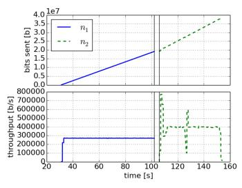
Figure 8: Throughput and total bits sent, registered at the 3 CARMNET nodes during the seamless handover experiment.
