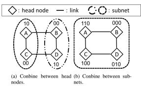
Figure 3: Group ID assignment procedure.
