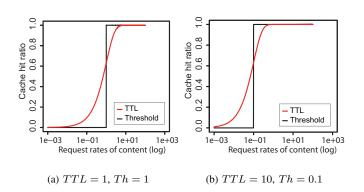
Figure 11: Comparison of cache hit ratio at a CR with threshold-based caching and TTL-based caching
