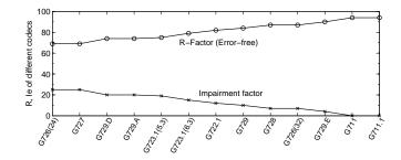
Figure 11:  $I_e$  and R-factor after compression.
