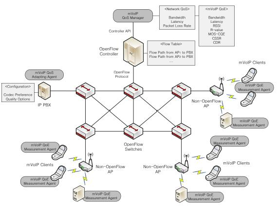
Figure 1. Adaptive mVoIP Service Architecture in SDN Networks
