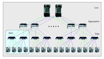
Figure 3- Typical network topology of a datacenter [5].
