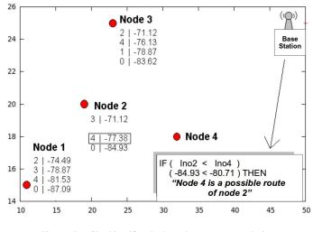
Figure. 5. Checking if node 4 can be a route to node 2.
