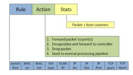
Figure 2. The OpenFlow Flow Entry [11]
