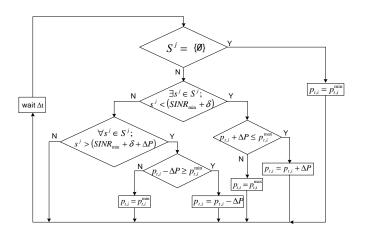
Figure 3. Flow chart of proposed power control algorithm.
