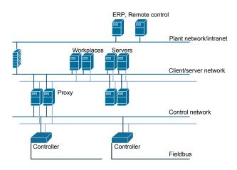
Fig. 1. An example of automation network architecture
