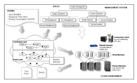
Figure 2 - Green Cloud management system based on OTM [6].
