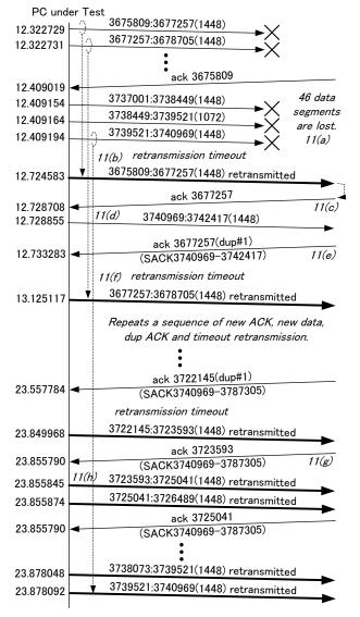
Figure 11. Timeline of segment exchanges at OS X (2)
