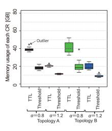
Figure 15: Box plot of memory usage for TTL-based caching and thresholdbased caching
