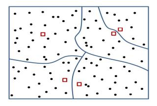
Fig. 1: An example of CHs and CMs arrangement in the LEACH algorithm.
