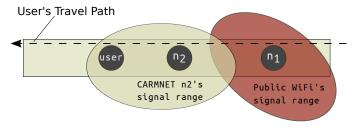
Figure 5: Network coverage extension experiment topology. Note that node  $n_1$ 's signal range has been omitted for clarity.
