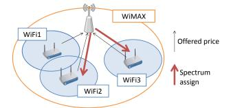
Figure 3: Channel assignment
