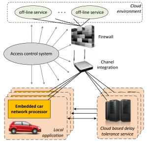
Figure 1. ITS system structure.
