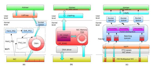
Figure 2. Adviser capturing packets (a) with NAPI and LibPcap (b) with PF\_RING (c) with PFQ.
