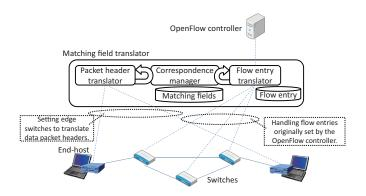
Figure 4. The architecture of the matching field translator.
