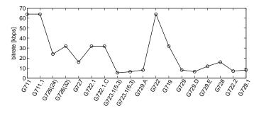
Figure 1: Raw bitrates of codecs.
