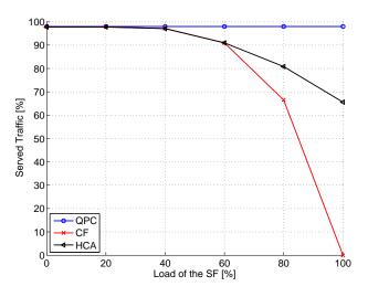
Figure 9. The amount of served traffic for FUEs depending on the load of the SF bands.
