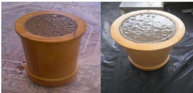
**Figure II.5: Essai de ressuage.**
