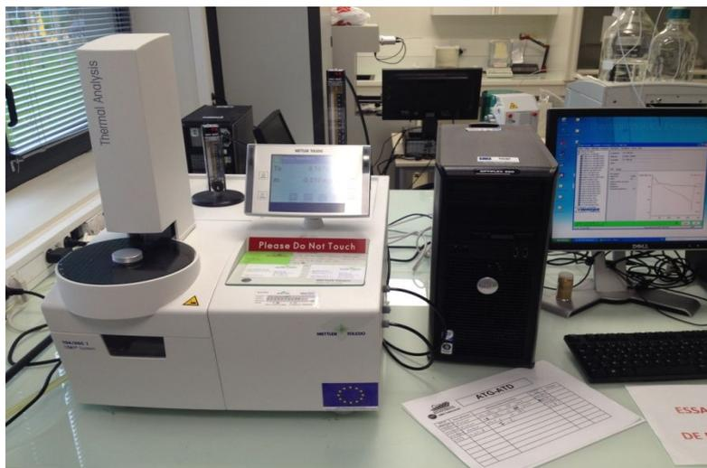
**Figure II.4: Appareil ATG Appareil METTLER TOLEDO TGA/DSC**
