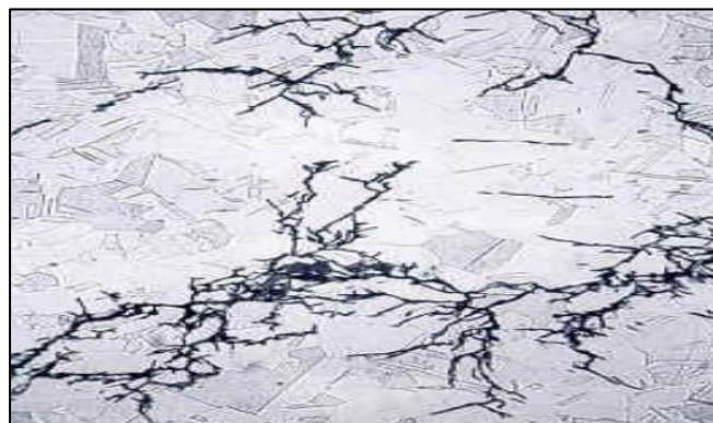
Figure II.8: La Corrosion inter-granulaire.
