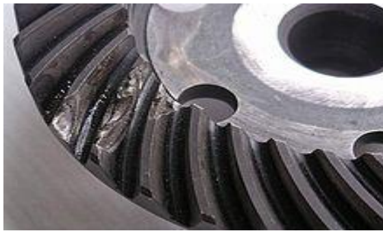
Figure 15 : Fissuration la denture.
