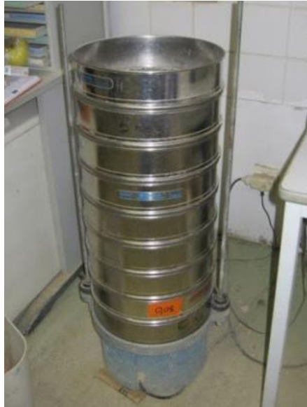
Figure IV.3: Essai de tamisage
