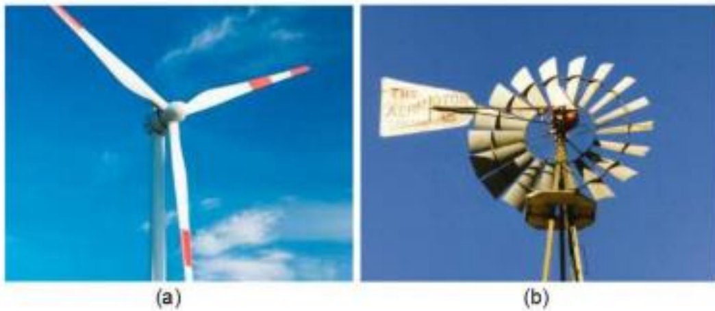
Figure II.19. Horizontal axis wind turbines: (a) three-bladed, (b) multi-bladed
