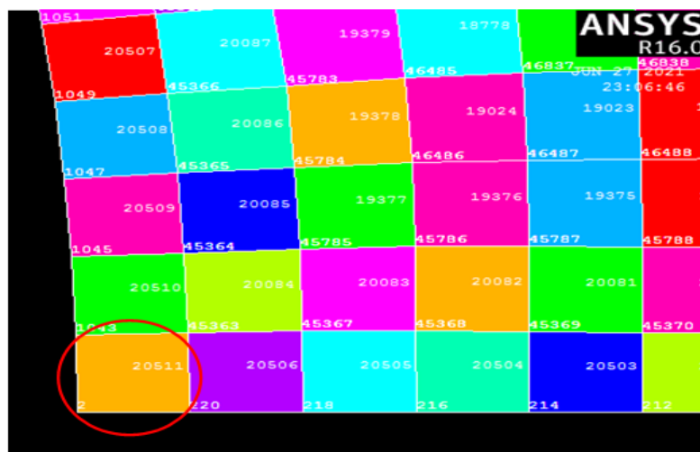
Figure III.10 Position de l'élément (20511)
