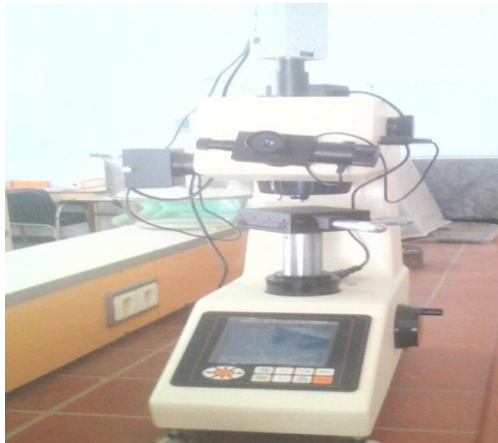
Figure III.7. Photo du micro dureté Digital Micro Vickers Hardness Tester.
