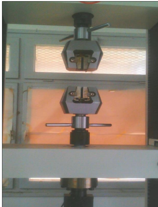
Figure III.4. La machine de traction.
