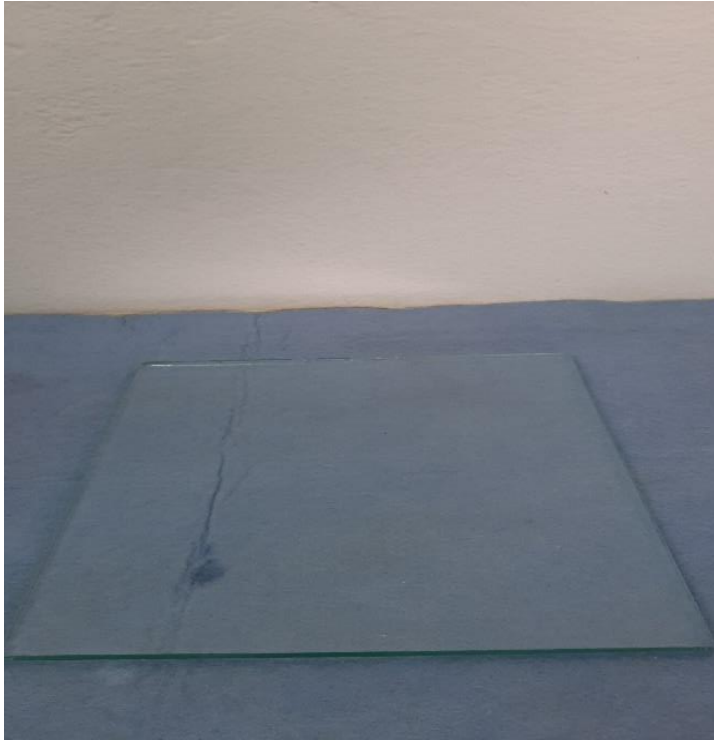
Figure 2-7. Flat glass plate for dope solution application
