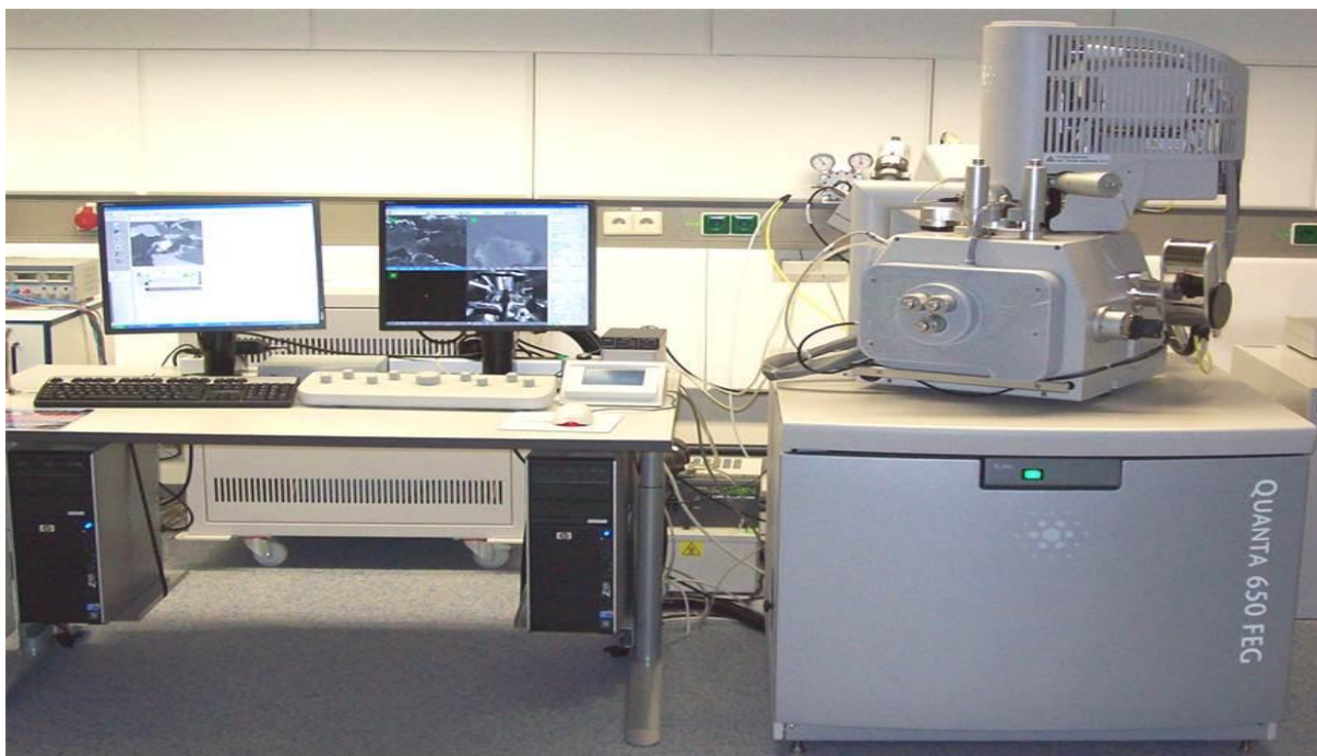
Figure 2-17. FEI Quanta 650 FEG SEM equipped with an EDS analyzer (Bruker QUNATX EDS XFlash® 6|10)
