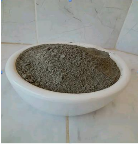
Figure II. 1: 450g de ciment
