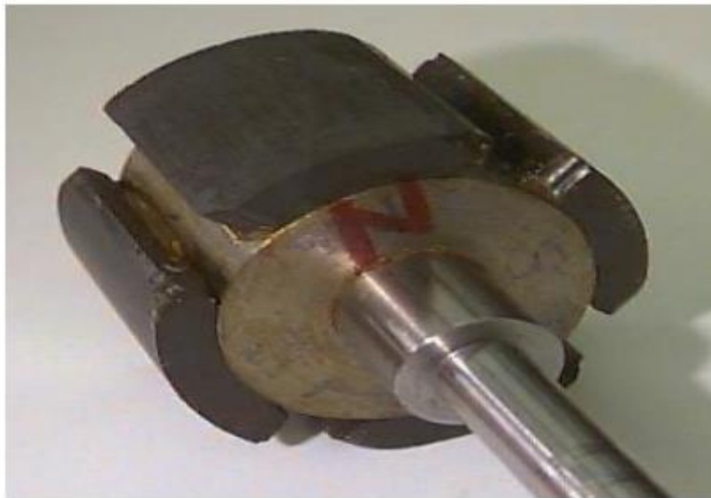
Figure I-8: Rotor d'une machine synchrone aimant permanent [7]
