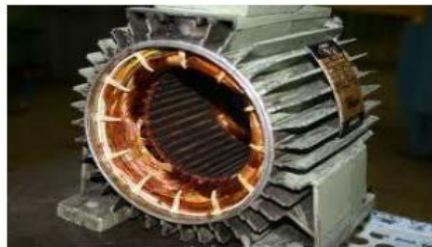
Figure I-7: Stator d'une machine synchrone
