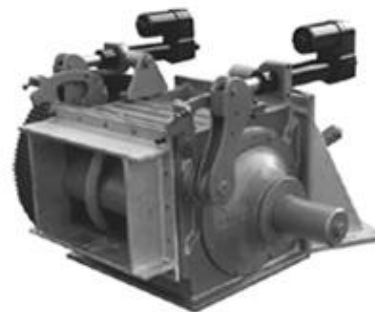
Figure I-18 : La turbine Banki ou Crossflow [22]
