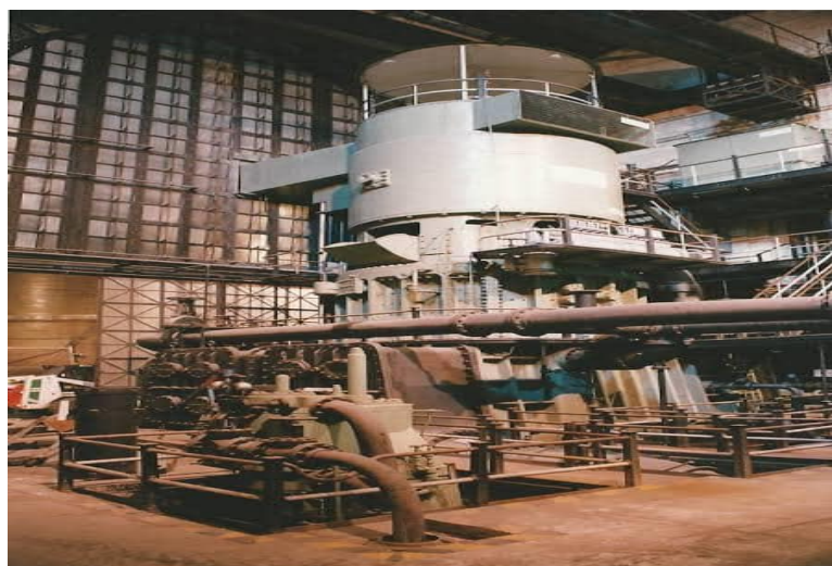
Figure II.5: Turbine Curtis a axe vertical [21]
