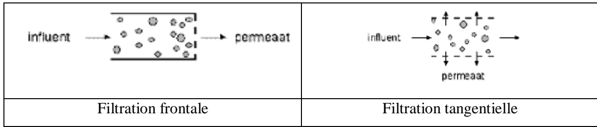
Figure II.4. Filtration frontale & filtration tangentielle
