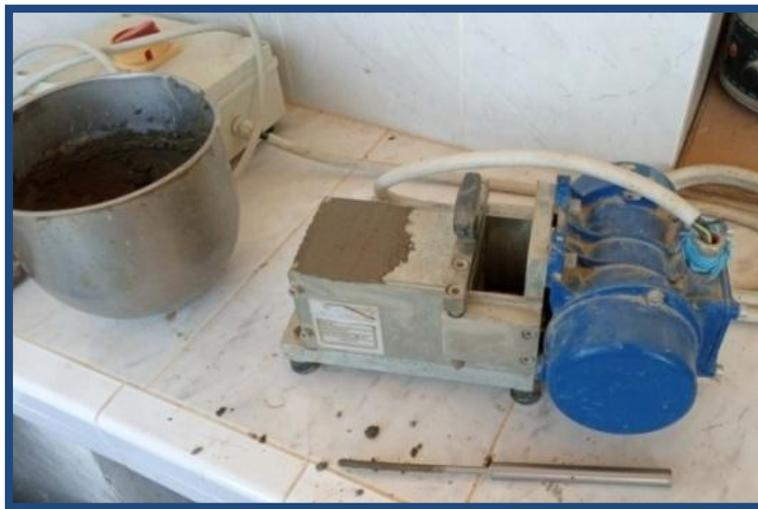
**Figure 5. 2-** Maniabilimetre type B.
