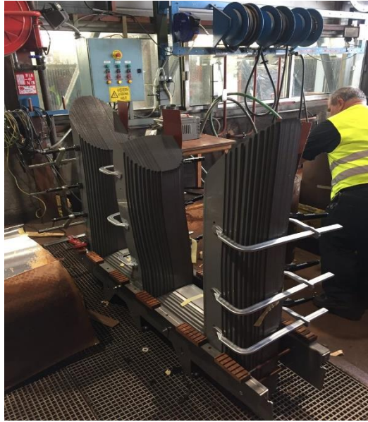
Figure 1. 12: The magnetic circuit of transformer
