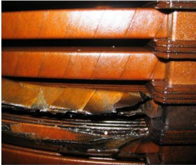
Figure 2. 6:Dielectric ignition between turns
