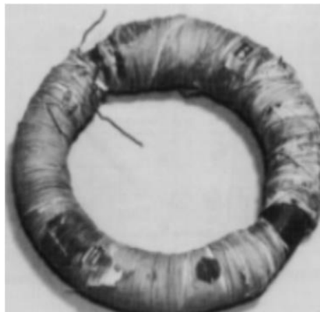
Figure 1. 4:Faraday's first transformer
