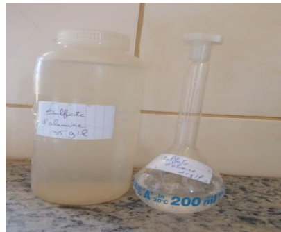
Figure 5-2: solution de sulfate d'alumine
