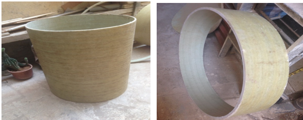
Figure II. 3. Pipelines en composite sandwich [15]
