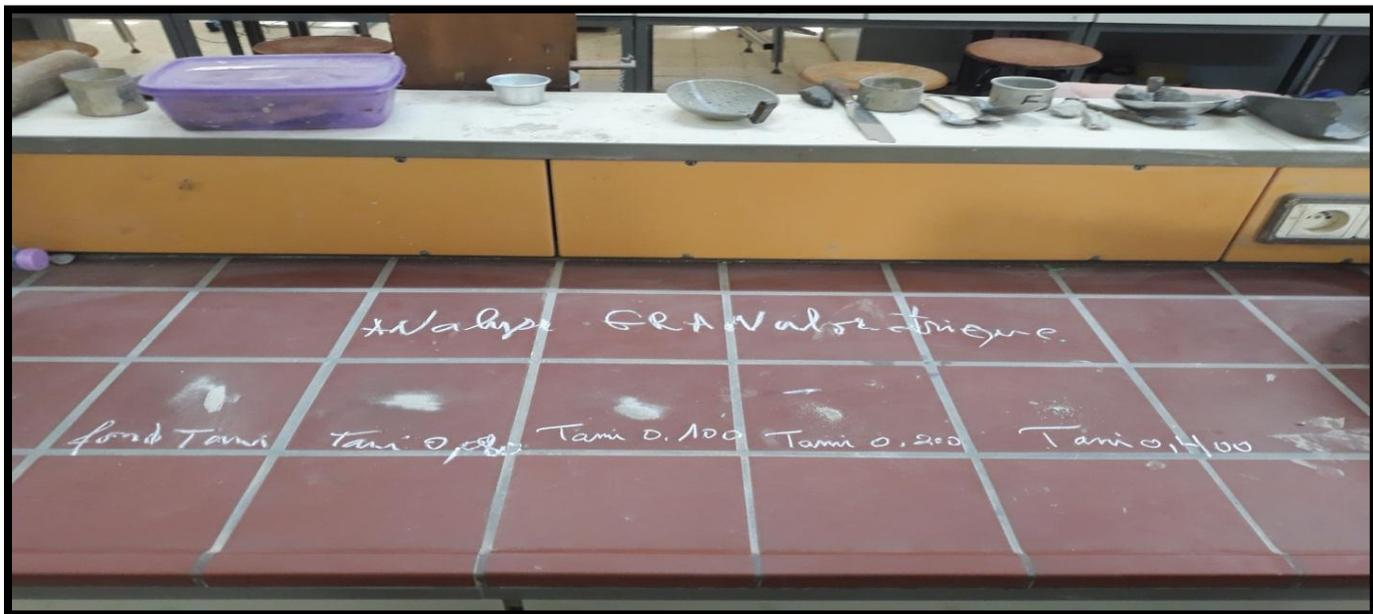
**Figure III.10.** Tamisage Fraction  $80 \mu\text{m} - D_{\text{max}}$ .
