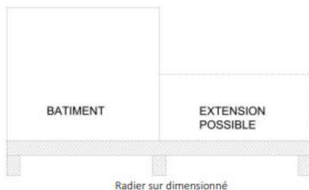
Figure 48 semelle évolutive source bazaed Architecture évolutive / flexible XB Architectes - Version 1 – 16/11/2015
