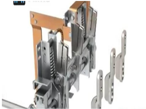
Picture II.23 : Earthing switch of the vacuum circuit breaker for all three phases.
