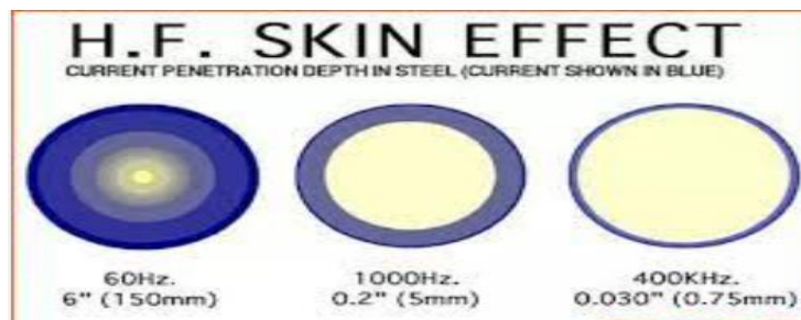
Picture I.4 : Skin effect as per the change on the frequency.
