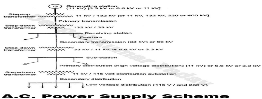
Picture I.1 : Drawing showing the path of electric power from production to exploitation.
