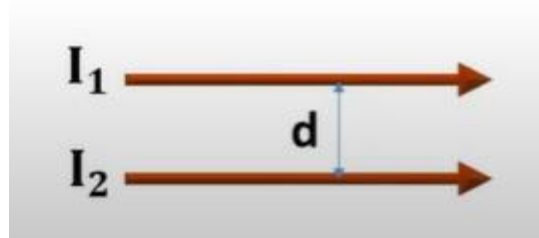
Picture IV.2 : Distance between two conductors
