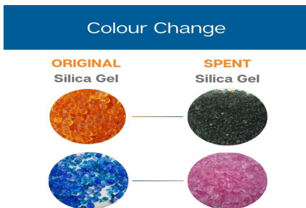
Picture III.12: silica gel status before and After use
