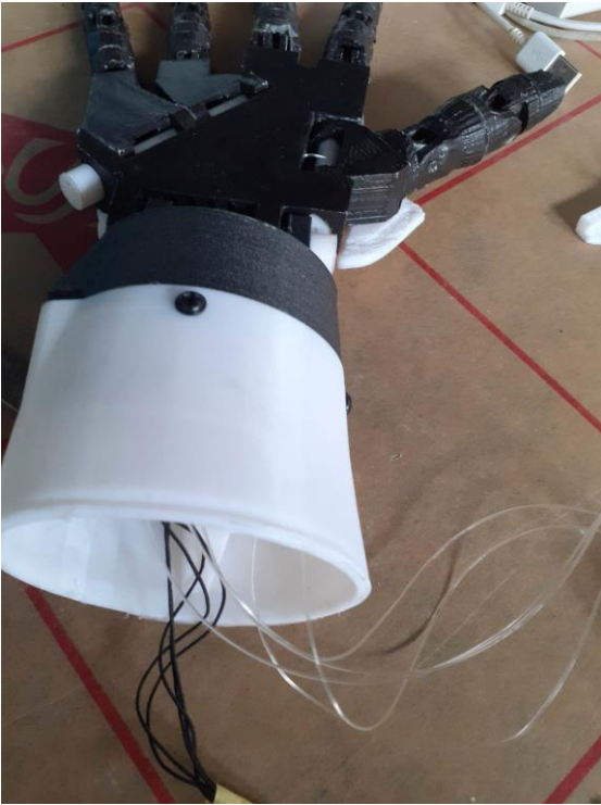
Figure III-5- Assemblage de la main
