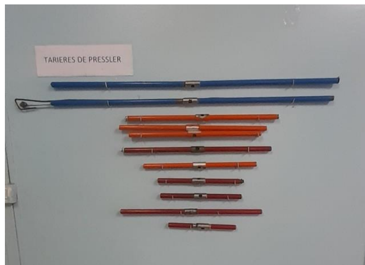
Figure 31. Tarières de Pressler
