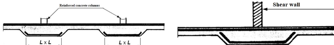
Figure 25 : Reinforcement of flat raft foundation to the right of the carrier elements
