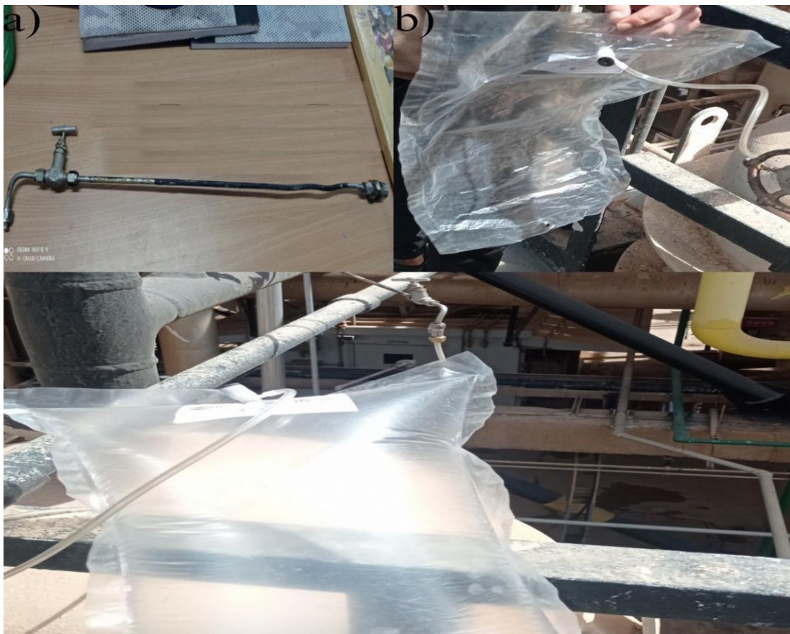
Figure II.1. Capture equipment, a) faucet with a pipe, b) sample bag.
