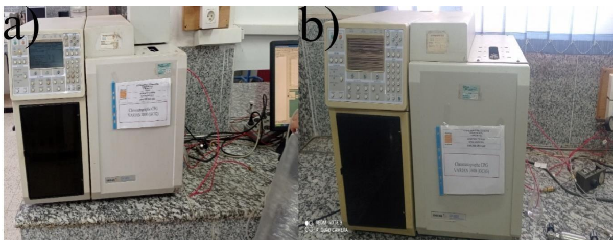
Figure II.2. Chromatograph (CP-3800), a) gas chromatograph 2 (GC02), b) gas chromatograph 3 (GC03).
