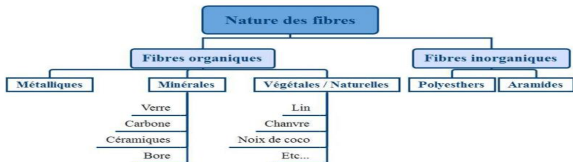
Figure I-7 : Types de renforts [15].
