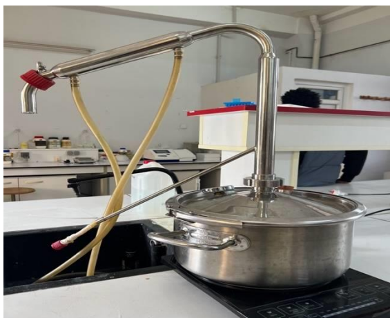
Figure 7: Schematic apparatus for Steam distillation
