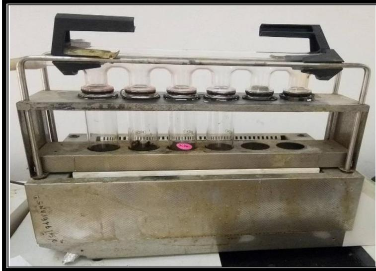
**Figure 22 :** Appareil de KJELDAHL
