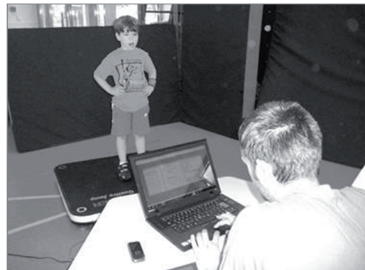
Figure 2. Vertical jump without arm swing (Countermovement Jump) at Kistler's Quattro Jump platform
