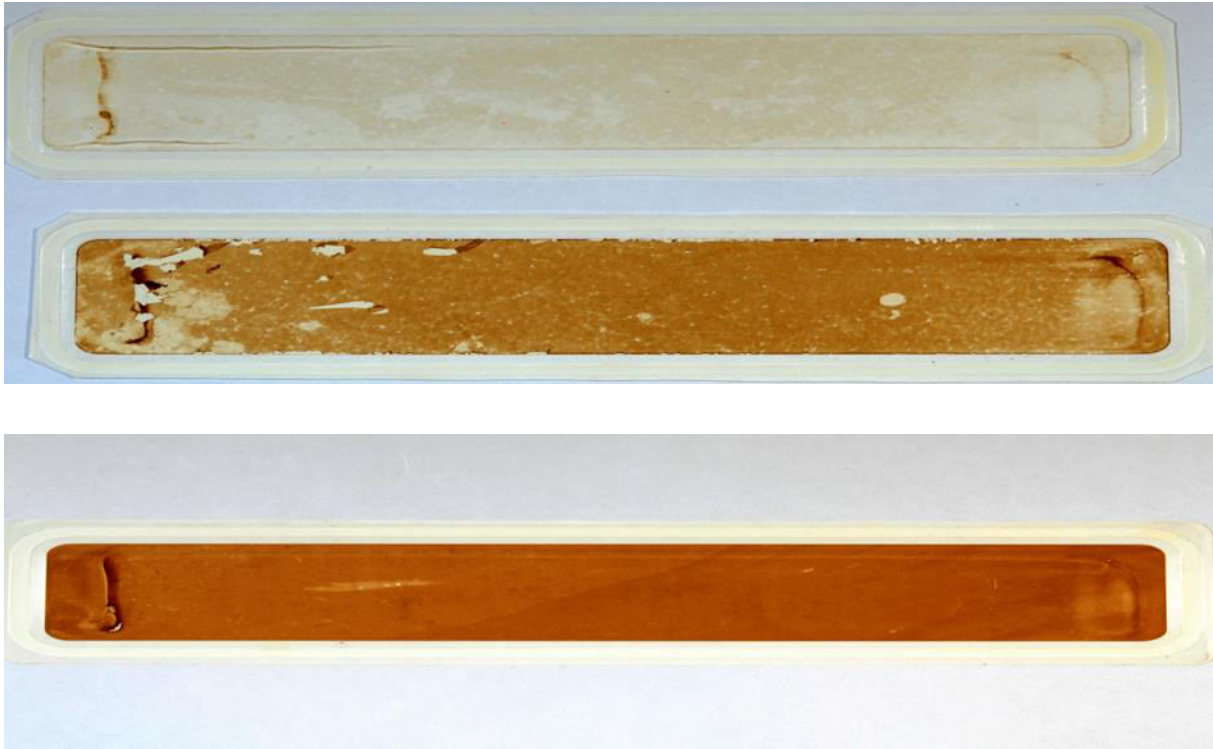
A.8. Resistance to humic acid fouling layer on membranes tested in the cross flow unit, Simatec.
