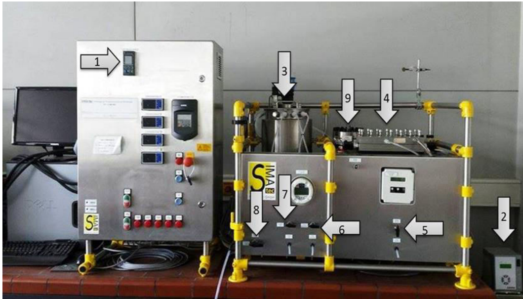
Figure.2.13. Experimental setup of the auto-controlled UF cross-flow testing cell. (1 pressure controller, 2 temperature controller, 3 feed tank, 4 membrane module, 5 permeate valve, 6 concentrate valve, 7 feed valve, 8 drain valve, 9 damping system)
