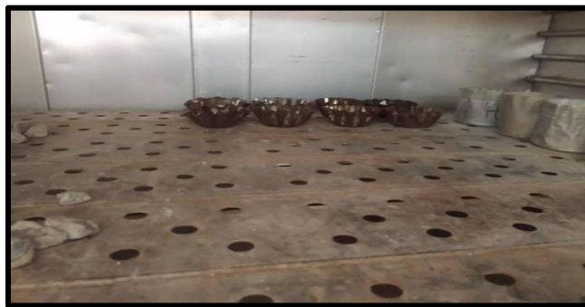
Figure (III.3) : Essai d'étuvage du sol
