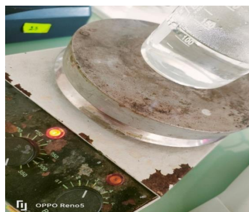
Figure 30: Heating of the solution of the organic matter
