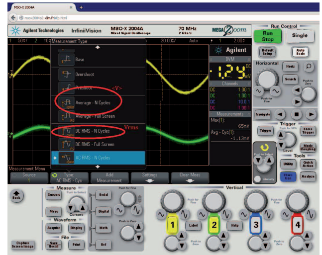
Fig. 3. Screenshot of the remote front panel of the oscilloscope. Each authenticated student connected to the application server can then monitor this oscilloscope as a face-to-face student.
