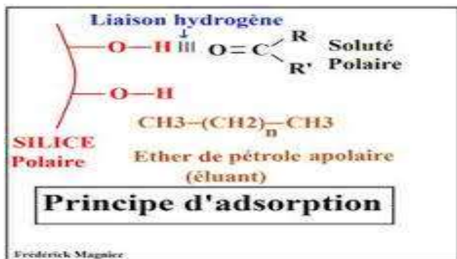
Figure 1. Principle of adsorption in silica chromatography
