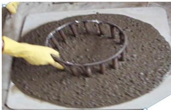
Figure III.4 : Aspect de l'essai J-Ring
