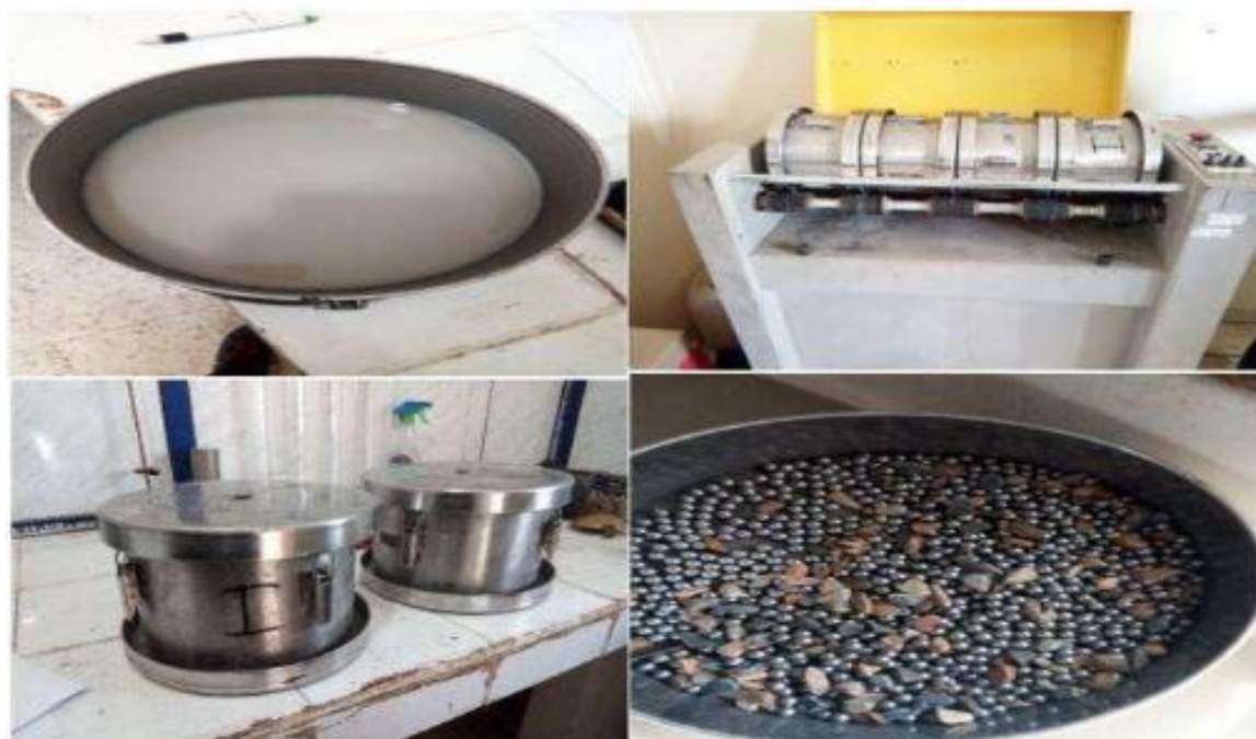
Photo II 8 : Essai de Micro-Deval
