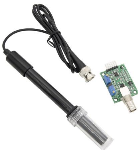
Figure II.6 pH electrode probe BNC with liquid pH between 0 and 14.
