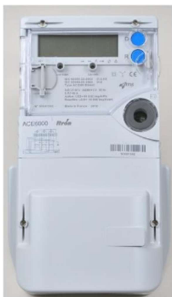
Figure 2.1: Front panel of the Itron ACE6000 electronic meter showing the LCD display, optical communication port, and metrological LEDs
