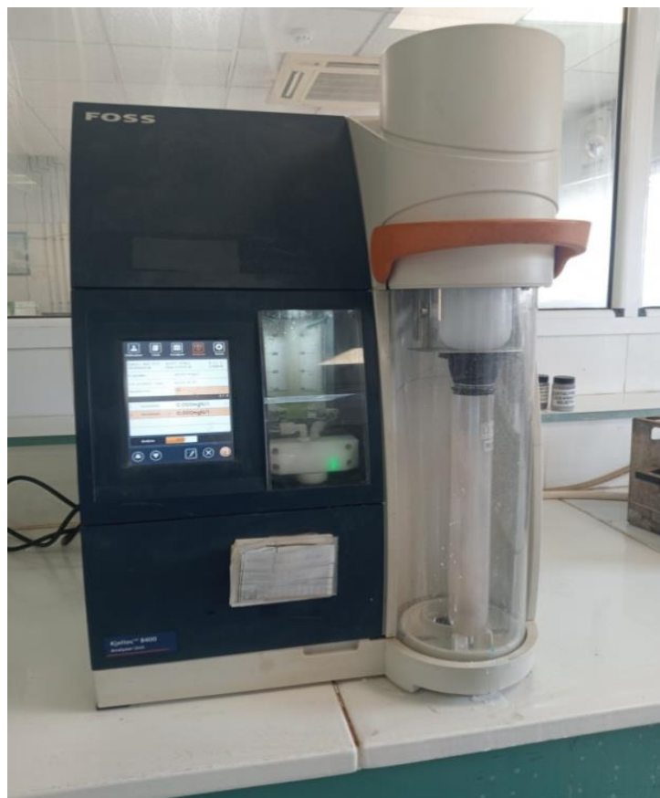
Figure III. 3: Appareil de distillation Kjeldahl
