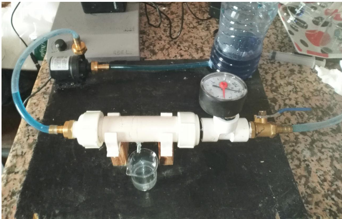
Figure III-14: Filtration system used to evaluate the performance of the ceramic membrane
