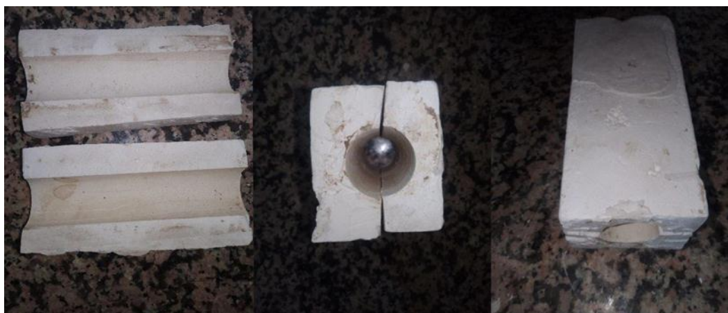
Figure III-7: Cylindrical mold made of gypsum for shaping ceramic membranes.
