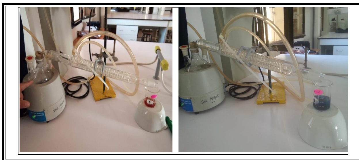
Figure 27: Distillation de l'ammoniaque
