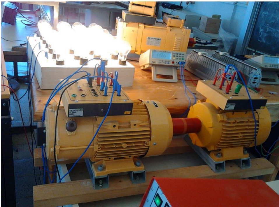
figure III- 4: essai en charge
