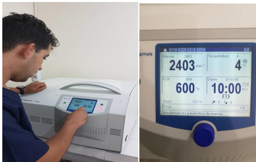
Figure 26 : Centrifugation a 600xg pendant 10min
