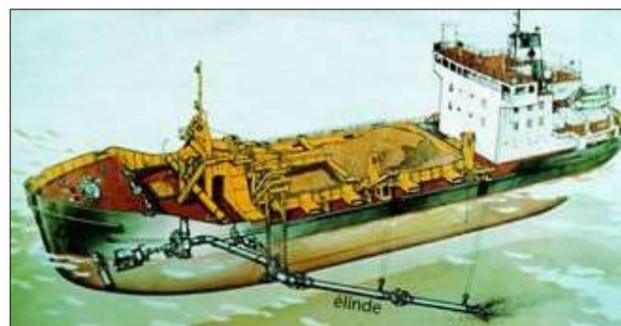
Figure II.12: Dragues aspiratrices simple [54].
