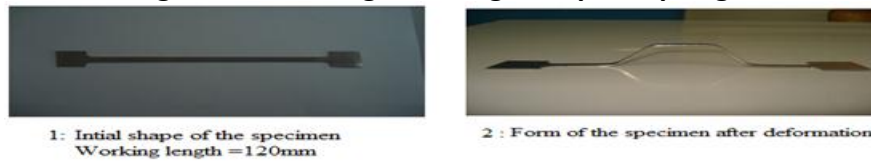
Fig.1.b, Form of specimen before and after unloading
