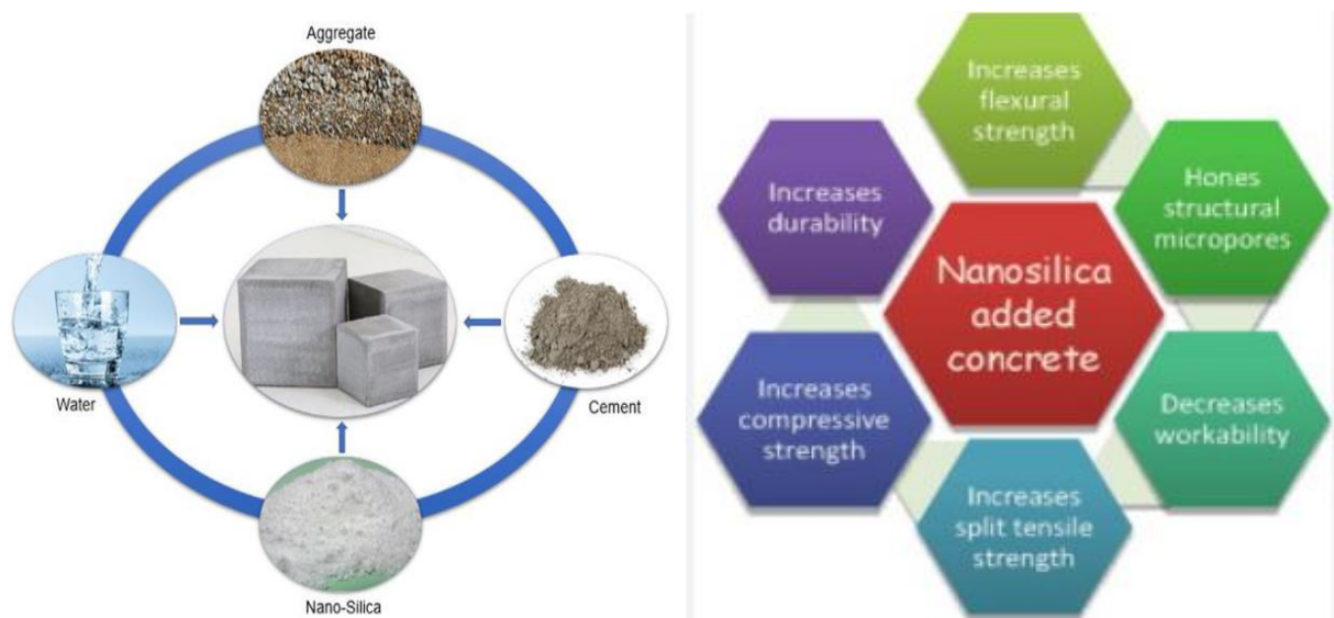
Figure I.5: Utilizing nano-silica in concrete exhibits advantageous enhancements, augmenting its overall performance and properties.[74]
