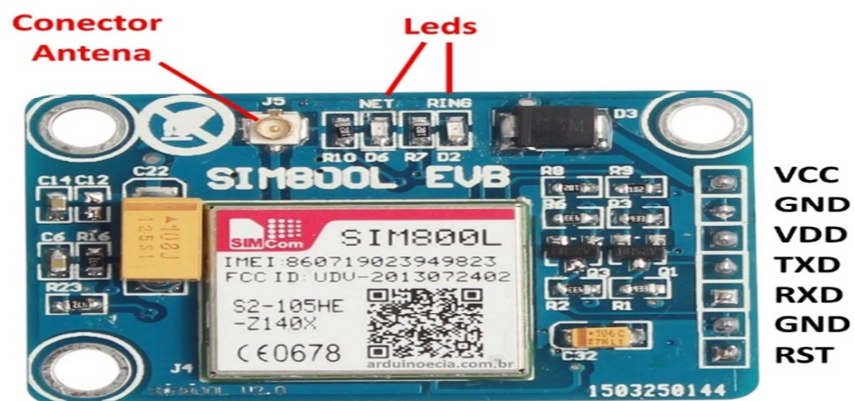
Figure II.3 : Module GSM SIM800L.
