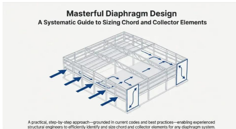
Figure 1: Load transfer mechanism in floor diaphragms.
