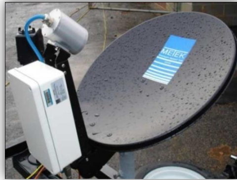
Figure I.15 : Micro Rain Radar (MRR) [15]
