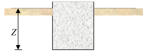
Fig.VIII.8: Encrage de la structure
